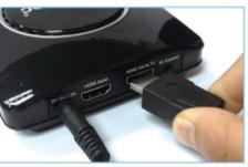
**Step 1c** Otherwise, get an HDMI cable from MyWirelessTV 2 Kit. Plug one end into the **HDMI Input** port on the back of the Transmitter.
