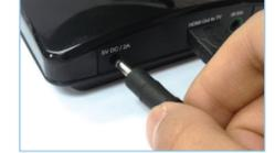
**Step 4b** Plug the larger end of the power supply into a power outlet.
