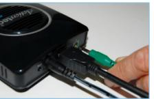
**Step 6c** Remove the protective covering of the double stick tape and attach the flat end of the IR Extender cable to the front corner of the HDTV bezel or frame.
