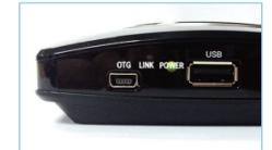
**Step 4d** Wait for a bit as the Receiver connects to the Transmitter. The LINK light should show SOLID Green once they're connected.
