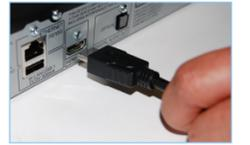
**Step 2a** Get the power supply from MyWirelessTV 2 Kit. Plug the smaller end of the power supply into the 5VDC port on the back of the Transmitter.
