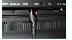
**Step 3c** Plug the other end of the HDMI cable into the HDMI port labels **Out-to-TV** on the back of the Receiver.
