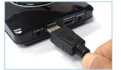
**Step 1d** Plug the other end into the HDMI port on the Source Device.
